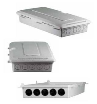
Enclosure includes two electrical knockouts on the bottom and five 2" (51mm) cable knockouts on top. 2" rubber grommets are available as an accessory item.
