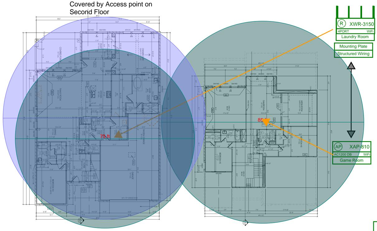
Note: 2.4 GHz WiFi coverage is guaranteed throughout the livable/ conditioned portions of the structure. Varying building materials and obstructions will cause significant degradation in the WiFi signal external to the structure. Thusly this map is not representative of actual external coverage to the home or structure and not covered under our WiFi guarantee.
