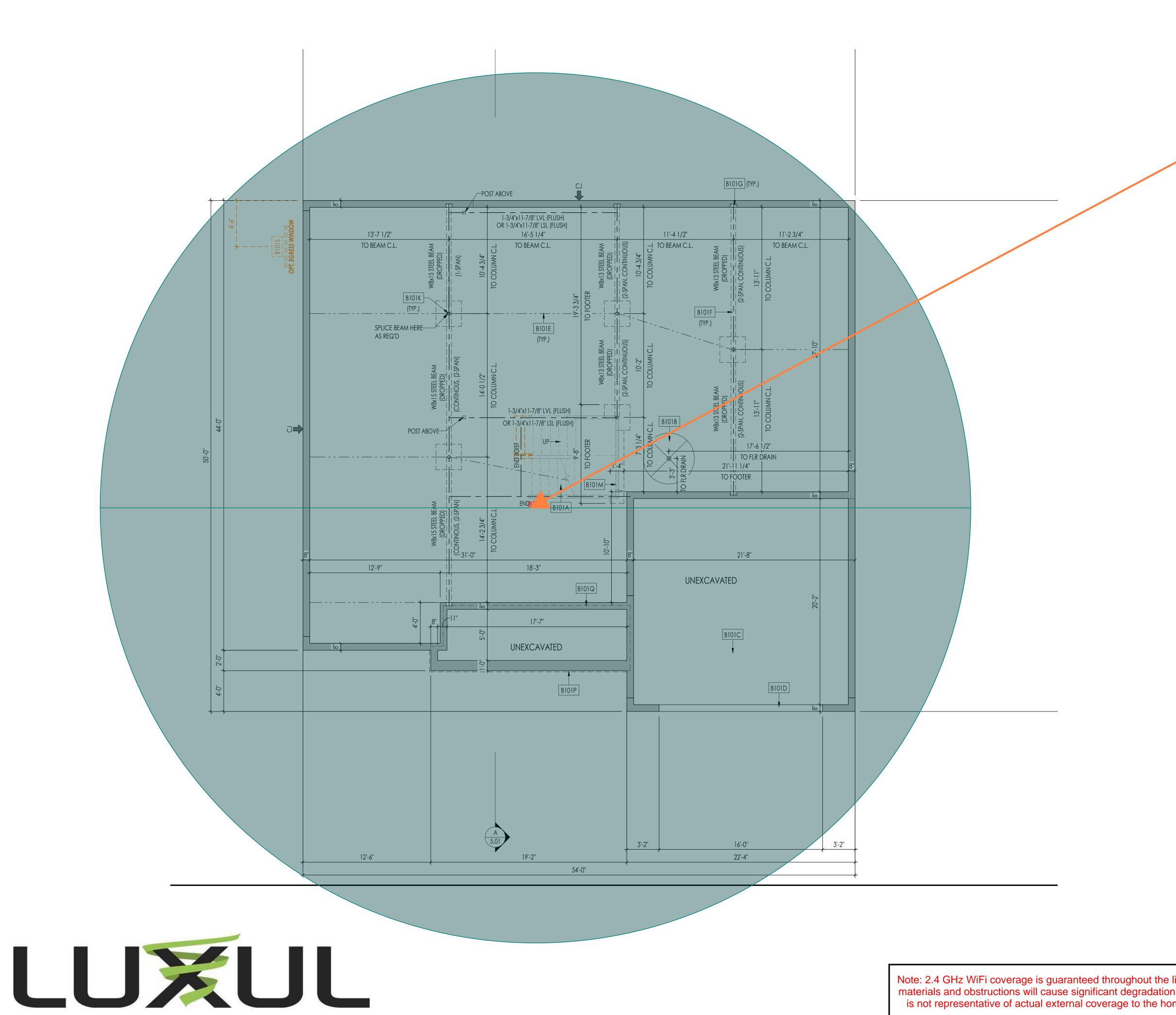
Note: 2.4 GHz WiFi coverage is guaranteed throughout the livable/ conditioned portions of the structure. Varying building materials and obstructions will cause significant degradation in the WiFi signal external to the structure. Thusly this map is not representative of actual external coverage to the home or structure and not covered under our WiFi guarantee.
