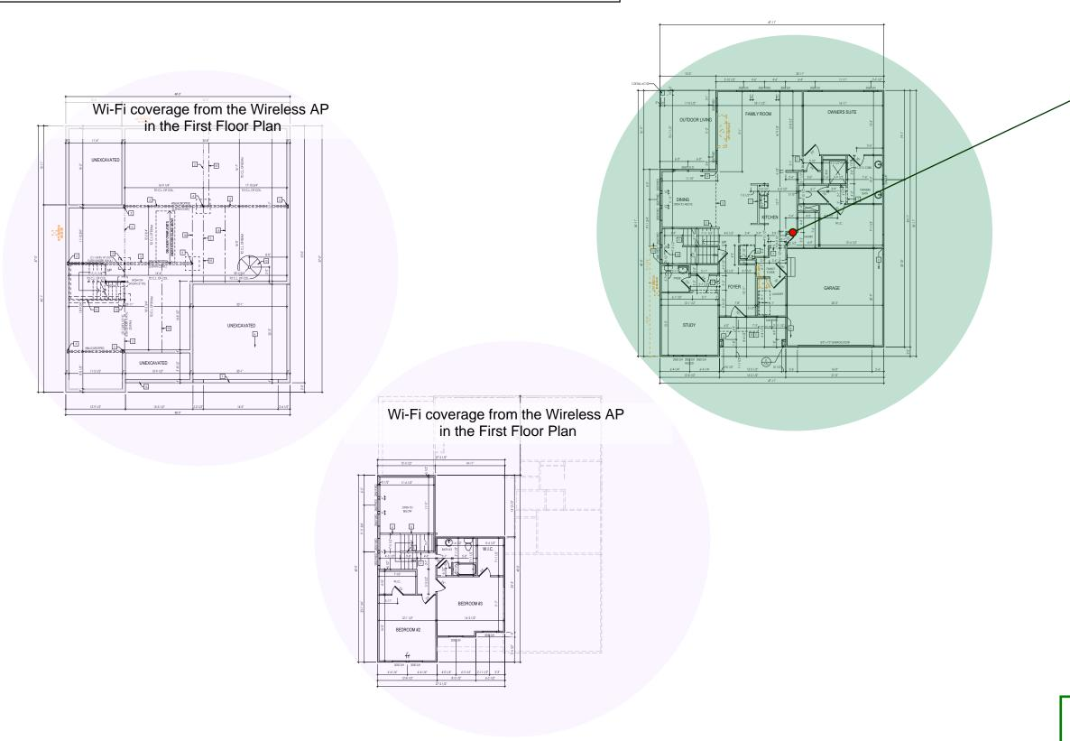
Note: 2.4 GHz WiFi coverage is guaranteed throughout the livable/ conditioned portions of the structure. Varying building materials and obstructions will cause significant degradation in the WiFi signal external to the structure. Thusly this map is not representative of actual external coverage to the home or structure and not covered under our WiFi guarantee.
