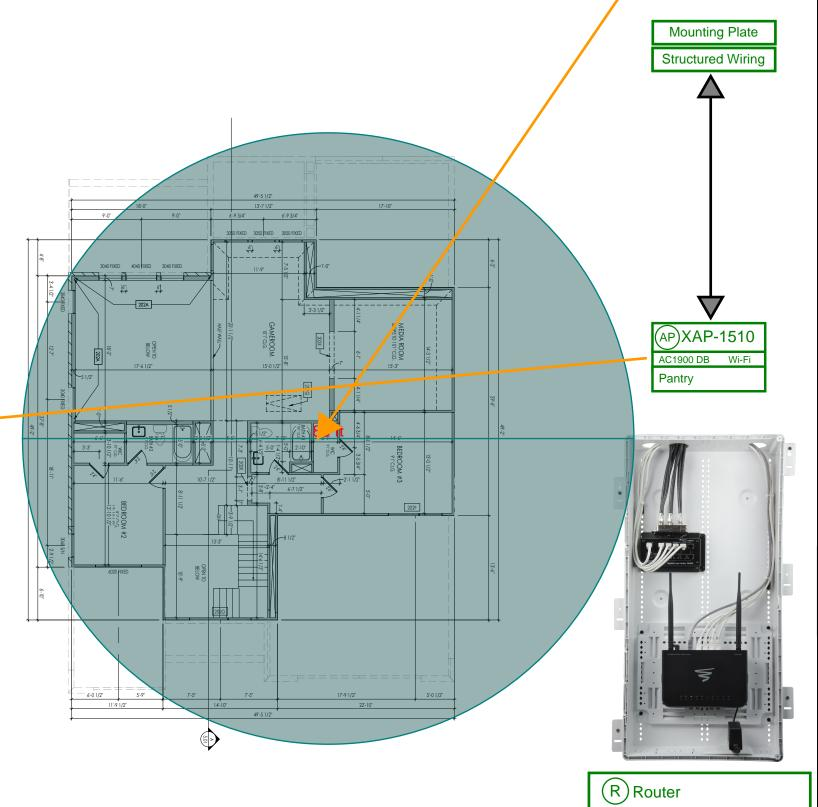
Note: 2.4 GHz WiFi coverage is guaranteed throughout the livable/ conditioned portions of the structure. Varying building materials and obstructions will cause significant degradation in the WiFi signal external to the structure. Thusly this map is not representative of actual external coverage to the home or structure and not covered under our WiFi guarantee.
